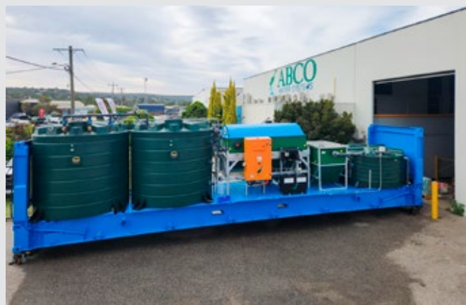
The portable mobile wastewater treatment system was built in Australia for rental purposes.
